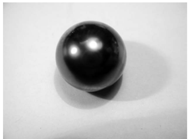
Figure 2 A 32 mm diameter TiN-coated Ti-6Al-4V femoral head (PIRAC, 900 °C, 4 h) after 4 \times 10^6 cycles of hip simulation tests in distilled water, at 2 MPa.
