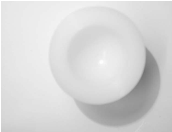
Figure 5 An UHMWPE cup after 4 \times 10^6 cycles of hip simulation tests in distilled water, at 2 MPa.
